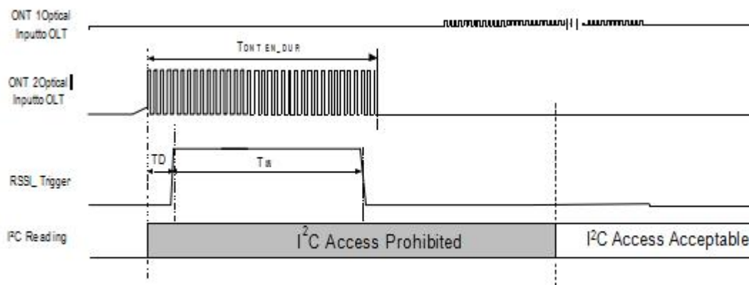
Figure 3 RSSI Timing Diagram
